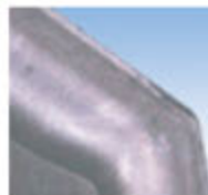
Abrasion on rake face
